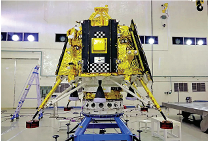
Figure 4: The Vikram lander carrying Rover and payloads
